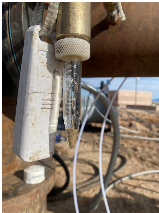
Total sand after 48 hours of pumping.
